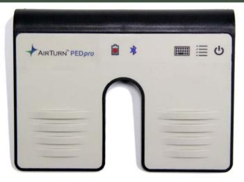
ON - Press and hold the Power Button on for one second and the LED's flash.
